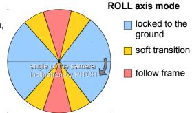
• **Follow YAW** – the same as above, except it can be used separately only for YAW axis. For example, you can lock camera by ROLL and PITCH axis by selecting "Disabled" option, but still control camera by YAW by enabling "Follow YAW" option.
