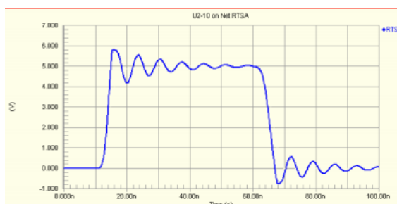
Bad signal (direct connection) and good signal (with resistor in series)
