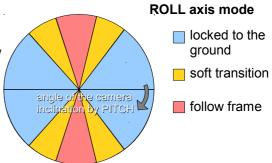
**Hint:** to completely disable follow for ROLL, set these values to (90, 0). To permanently enable follow for ROLL (regardless of the camera PITCH-ing), set values to (0, 0).
