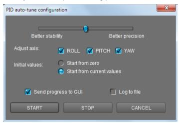
Slider at the top defines the target of tuning. If its close to "Better precision", it will try to achieve maximum gain and keep it. If close to "better stability", it will find maximum gain and than decrease it by 30-50% to make system more stable.
