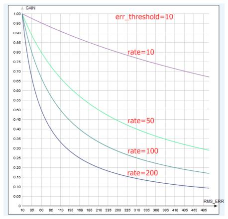
• Recovery factor, 0..10 - defines, how fast PID gains are recovered back when the system becomes stable. Too low value may increase a chance that vibration comes back in short time. Too high value may cause worse operation (because lowered PID values are kept longer). Recommended value is 5..6
